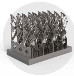
Full Substrate Braced Frame
